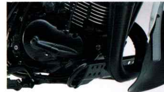
Functional engine guard bar and plate
